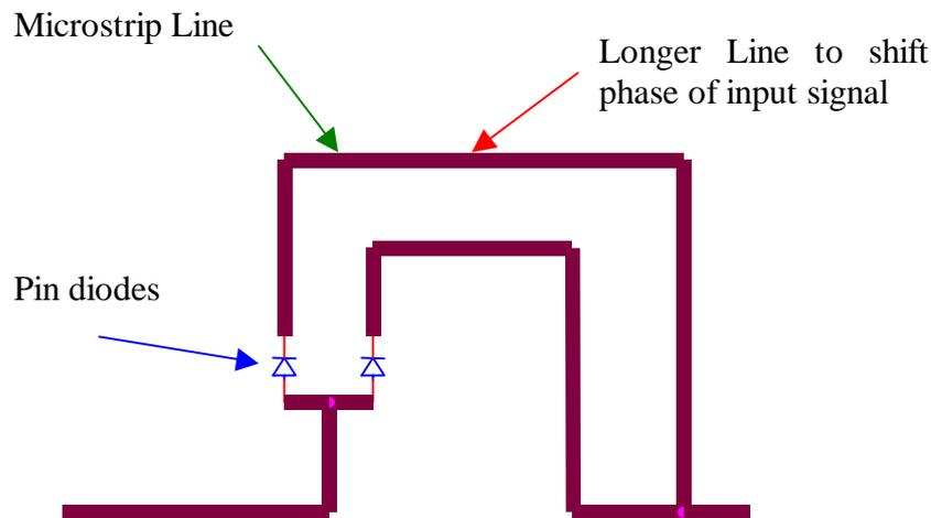
The upper transmission line is longer than the lower line by  $45^\circ$ . Thus if applied to an array I would have achieved our required phase shift to an array in order to steer the beam.
