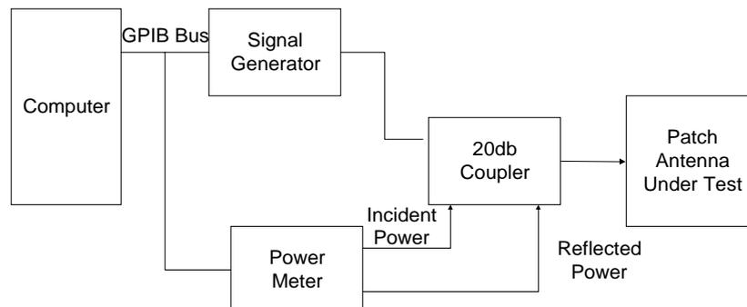
The signal generator was swept through a range of frequencies. Channel A of the power meter was used to read the input power from the 20db coupler while Channel B was used to read the reflected power from the antenna under test. The reflection coefficient was calculated from this formula:
